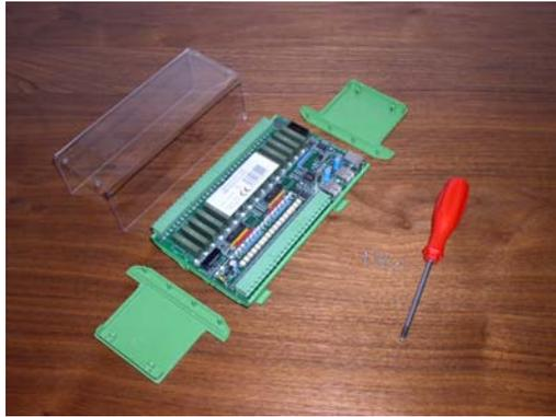
The lateral walls can easily be removed by gently pulling them free of the holding pins.
