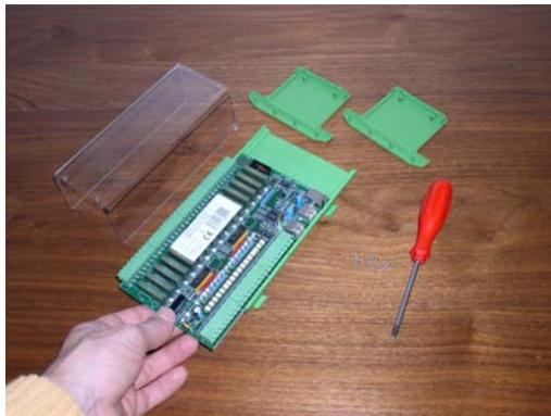
Now slide out the board from the plastic mounting rails.
