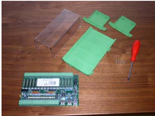
The USB-I/O is fully disassembled in all its parts.
