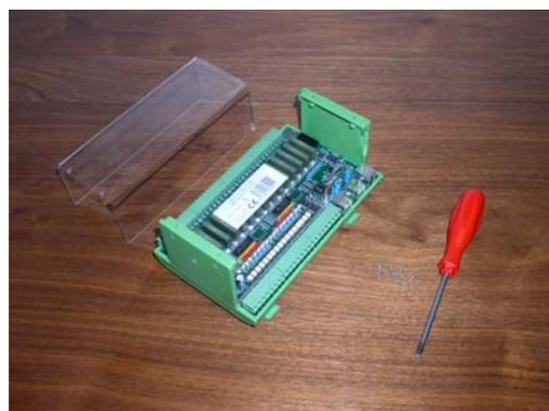
Now carefully remove the protective cover. Of course be careful not to lose track of the removed screws or of the other disassembled parts!
