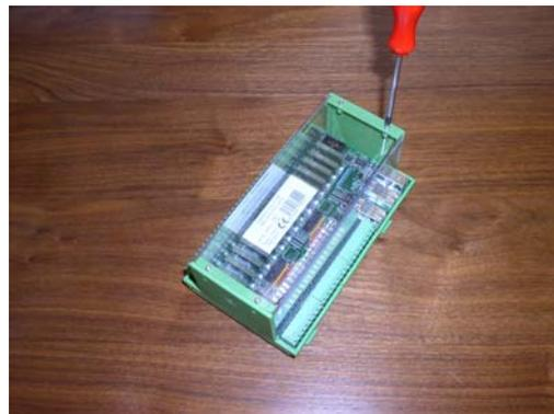
Remove the 4 self threading screws that hold the transparent protective cover.
