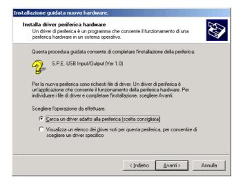
6) According to the USB-IO board type select the right .inf file from the operating system specific directory in the installation CD.cegliere l'opportuno file .inf dalla directory drivers del CD di installazione.
