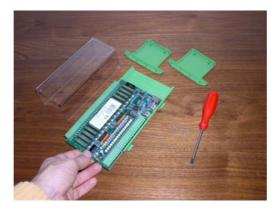
Now slide out the board from the plasting mounting rails.
