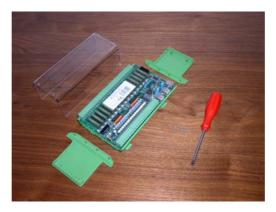
The lateral walls can easily be removed by gently pulling them free of the holding pins.
